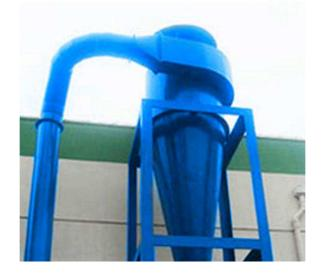
YDT type vertical multi-tube ceramic dust collector is made of 250mm standard ceramic cyclone circular arrangement, compared with the square, it has a simple structure, beautiful appearance, not easy to accumulate ash, small size, small footprint, Small resistance, low steel consumption, low cost, etc.
